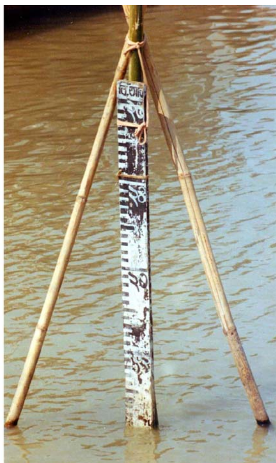
Water level gauge
